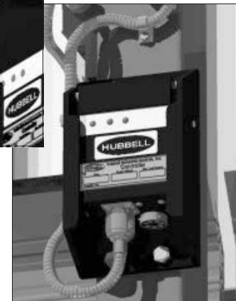
These illustrations show several remote mounted Infrared Hot Metal Detectors in use on a billet mill. The unit mounted on top of the stand is a 0.5° x 10° Cast Lens Housing and it is being used to measure the length of the slabs. A Tubular Lens Housing is mounted on the side of the stand and is measuring the rough heights of the slabs. Notice how the controller is mounted behind the stand to protect it from radiant heat.
