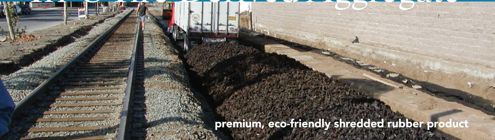
**Tri-C Tire Derived Aggregate (TDA)** is sized reduced California scrap tires used in various public work projects and civil engineering applications. **Tri-C**
